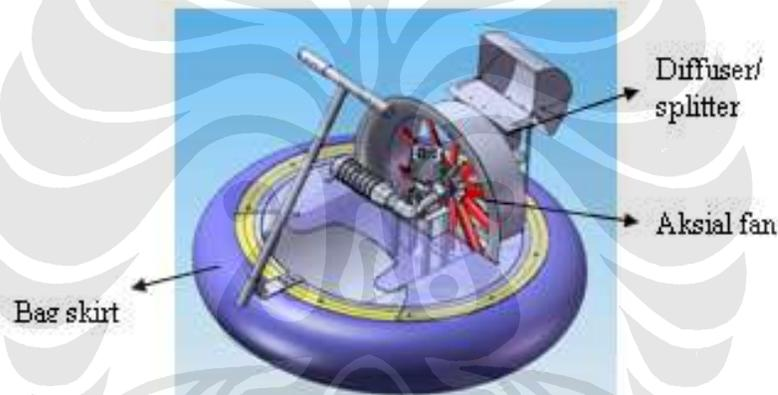
Gambar 3.2 Disain original *integrated circular hovercraft proto-X1*
