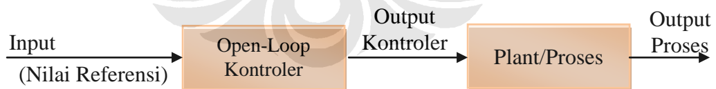
Gambar III. 2 : Diagram Blok Open-Loop Kontroler [7]
