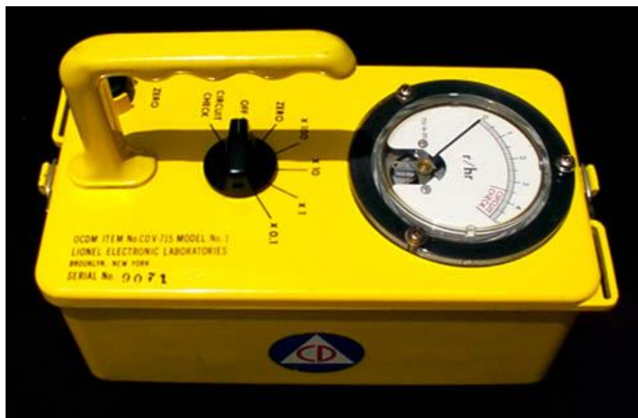
Civil Defense High-Range Survey Meter 0-500 R/hr range
