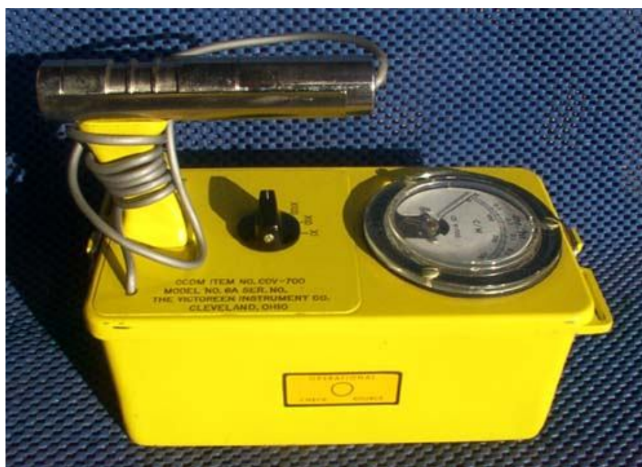
The detector on the CD V-700 is a Geiger-Mueller (GM) tube. It measures gamma radiation. It has a check source on the side and a headphone jack. The range selector switch allows you to measure up to 50 mR/hr. A milliroentgen (mR) is one thousandth of a Roentgen (R).
