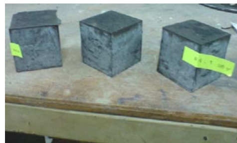
Gambar 4.2 Benda Uji Kubus 5x5x5 cm 3
