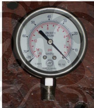
Gambar 3.4. *Pressure gauge* vakum
