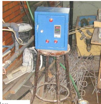
**Gambar 3.7 Heater Controller**
