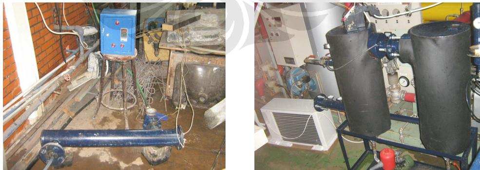
**Gambar 3.4** Alat uji *Throttling Process*
