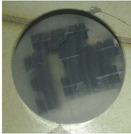
Gambar 3.4. Sampel aluminium foil hasil mounting melintang
